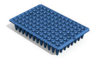
light frosted surface enables signal enhancement in qPCR
